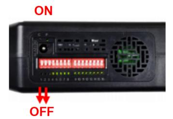
Once you've activated the Power Switch, make sure to also enable the DIP switch. The DIP switch is responsible for managing each individual antenna. Each number indicator corresponds to a specific antenna, and when the LED associated with an antenna is illuminated, it indicates that the antenna is operational.
