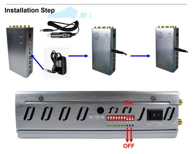
Once you've activated the Power Switch, make sure to also enable the DIP switch. The DIP switch is responsible for managing each individual antenna. Each number indicator corresponds to a specific antenna, and when the LED associated with an antenna is illuminated, it indicates that the antenna is operational.
